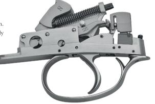
Z-Guns series trigger assemblies (Z-Expedition, Pernice and Custom line) have their critical parts Titanium Nitrate treated and the powerful main coil springs are coated with a self lubricating material for maximum corrosion resistance and minimum wear.
